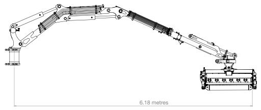
Working radius with extended sliding boom.\*
