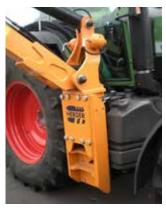
Pivot 'rotating cylinder' for narrow mounting.
