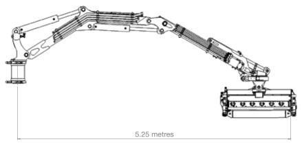
Working radius with retracted sliding boom.\*
