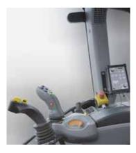
The joystick ensures accurate operation of the booms. Nivotronic is taking care of the adaption to the surface during work.
