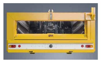
Special tank frame for the hydraulic tank keeps the top tow bar accessible for a trailer.
