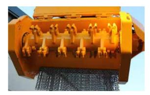
Close-up of rotor shaft with teeth
